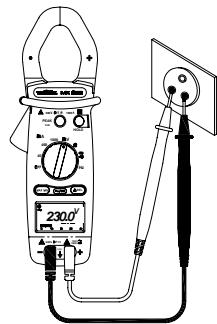
Connect the red test lead to the "+" input terminal and the black test lead to the "COM" input terminal.
