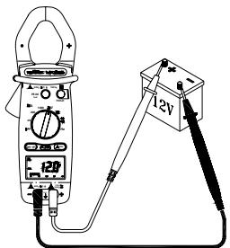
Press on the  $\sim/==$  button to display the  $==$  symbol (direct signal).
