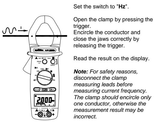
**Note:** To measure frequency, either the input terminals (voltage) or the clamp jaws (current) can be used, but the two sources should never be used at the same time.
